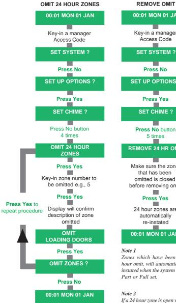
00:01 MON 01 JAN Key-in a manager Áccess Code **SET SYSTEM ? Press No SET UP OPTIONS ? Press Yes SET CHIME ?** Press No button 5 times **REMOVE 24 HR OMIT** Make sure the zone that has been omitted is closed before removing omit **Press Yes** 24 hour zones are automatically re-instated 00:01 MON 01 JAN
