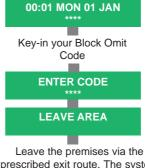
prescribed exit route. The system will automatically re-arm the circuits in Group 'D' on expiry of the exit timer or closing of the final door, or pressing the exit terminate button. (Refer also to Notes 3 & 4 Page 3)
