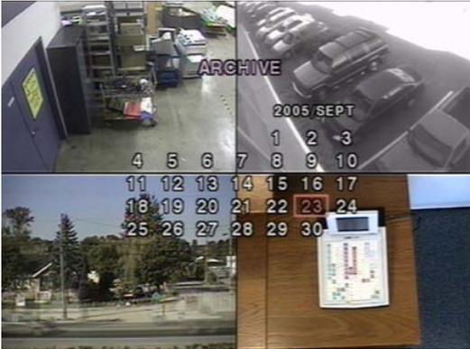
1. Select the date to begin searching by using the **LEFT**, **RIGHT**, **UP**, and **DOWN** buttons to navigate through the days.
