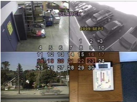
1. Select the date of the video to begin searching by using the **LEFT**, **RIGHT**, **UP**, and **DOWN** buttons to navigate through the days.
