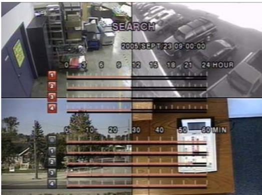
4. Select All or a specific channel to search by using the **UP** and **DOWN** arrow buttons. Notice that the highlighted icon on the lower left side of the screen changes when **UP** or **DOWN** is pressed.
