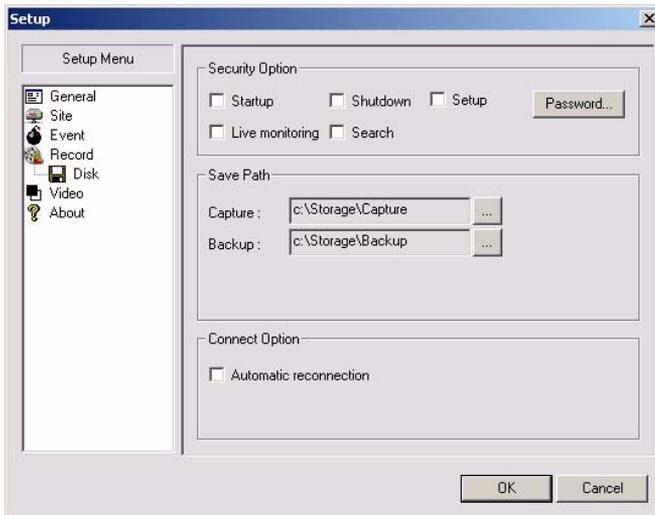
1. In the **Security Option** section, click the checkboxes to place a checkmark in those boxes. The options that you select will now require a password when a user accesses that function. The same password is used for all security options enabled.
