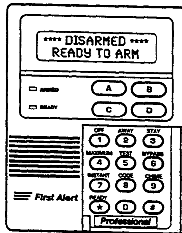
FA550KP Alpha Keypad (shown with cover removed)
