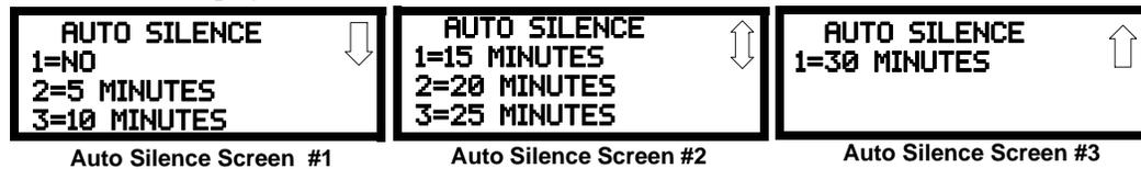
To disable the Auto Silence feature, press 1 for *No* while viewing Auto Silence Screen #1. To enable the Auto Silence feature, press the number corresponding to the time delay which will elapse before Auto Silence activates. This information will be stored in memory and the display will return to NAC Screen #1.
