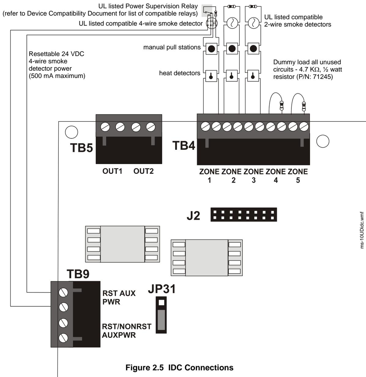
Figure 2.5 IDC Connections
