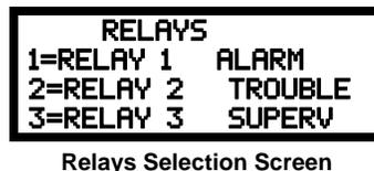
To program Relay 1, 2 or 3, press the number corresponding to the selected relay. The following screens will appear for each relay to be programmed:
