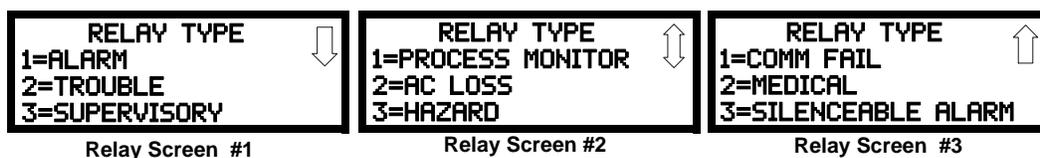
While viewing the selected screen, press the number corresponding to the desired relay type to program the main circuit board relay. The choice will be stored in memory and the display will return to the Relay Type Screen which will show the programmed type choice. Press the Escape key to return to the Relays Selection Screen and repeat the preceding procedure for the remaining relays.
